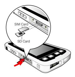
3. To remove a card, push the card to release from the slot.
